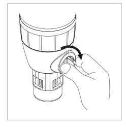
When the backwash operation is completed, turn the backwash knob anticlockwise by 90° back into the initial position.
