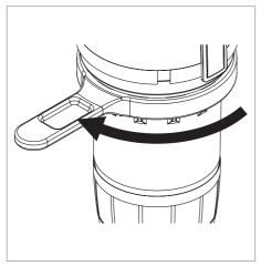
Remove the pressure reducer cartridge together with the suction casing and the suction pot by pulling out upwards. The spring remains in the filter cap.
