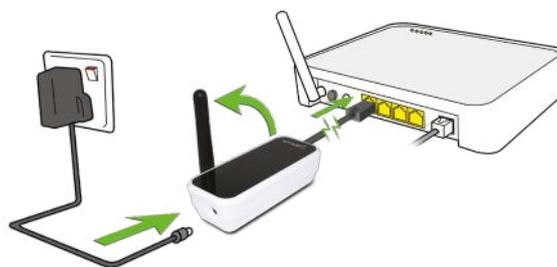
After connecting the gateway, the red LED should start flashing
