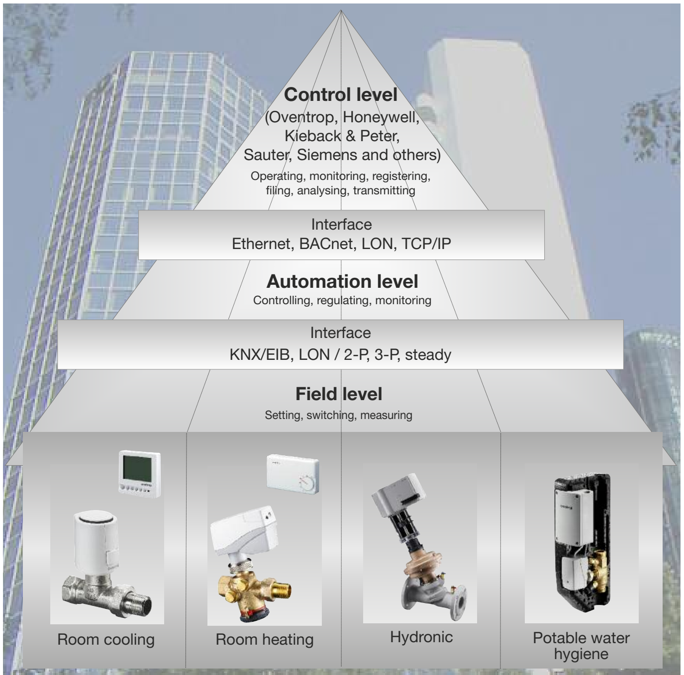
Overview building automation and system components
